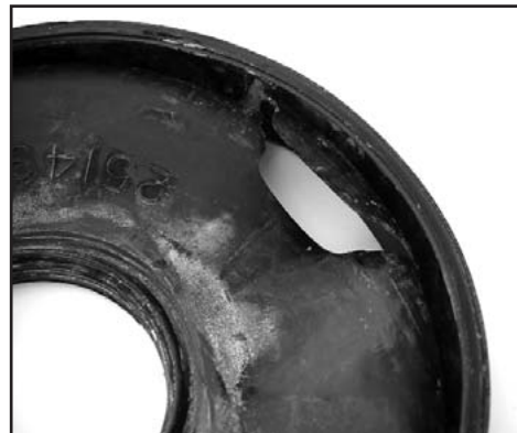
Typical vacuum booster diaphragm failure due to gas or gasoline fumes
