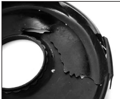
Typical vacuum booster diaphragm failure due to gas or gasoline fumes
